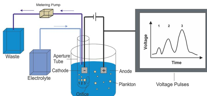
**Figure 2.** Schematic diagram of the Coulter Counter experiment showing how the plankton are in a suspension and are then pumped through an orifice. The change in the electrical resistance of the orifice leads to pulses in the voltage time profile as measured using the Coulter Counter. For a given particle shape, the magnitude of the pulse is proportional to the volume of the particle traversing the orifice.
