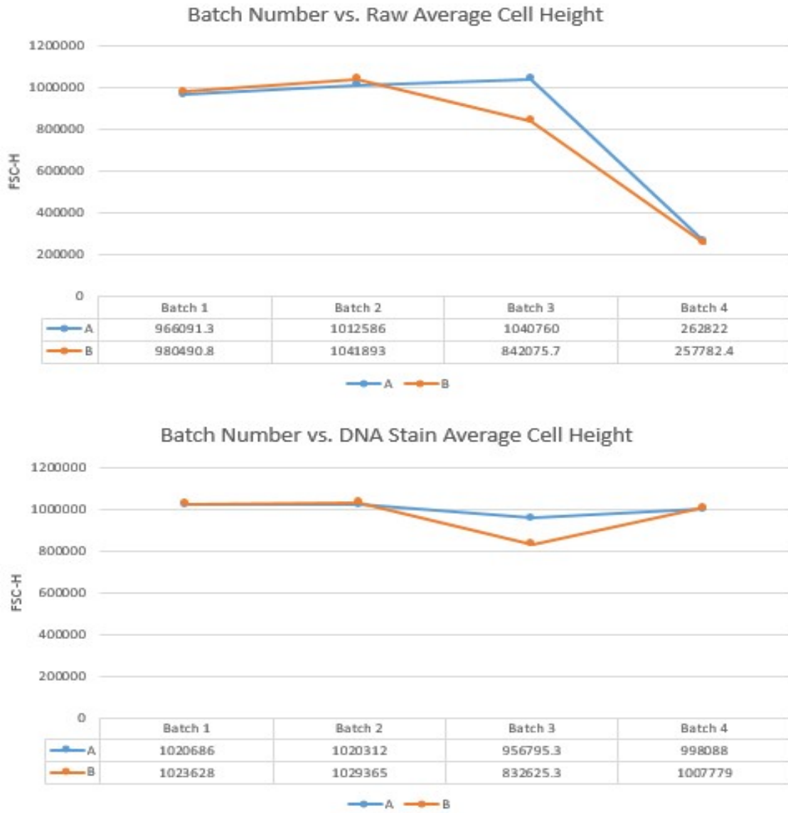
Figure 50 Average Cell Size per Batch both Raw and Through the DNA Stain for both A and B cultures.
