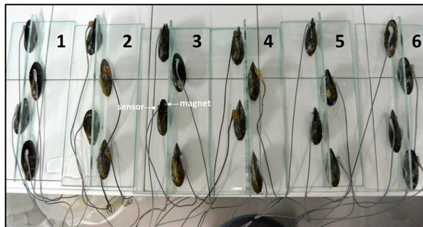
Fig. 1. Photo of 24 *M. galloprovincialis* individuals equipped with Hall sensors and magnets. Glass supports allowed byssus fixation.
